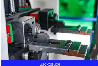
The overall structure is made of lightweight materials, providing high rigidity and fast speed. It comes standard with two CNC axis (X and R), and the backstop can move left and right along the cylindrical guide rails.
