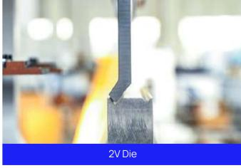
The lower die utilizes a double V quick-change clamping method, with an optional single V mechanical clamping system available.
