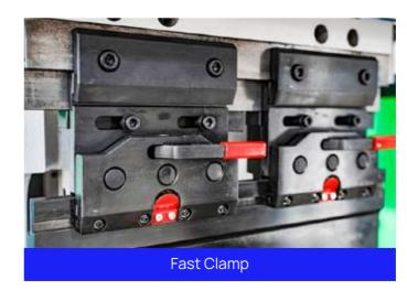
The standard configuration for the upper die clamping device is a mechanical quick-clamp system.
